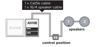
Each audio zone to be wired for multi-room audio will have a Cat5e + 4 core speaker cable run via a suitable control position (typically a switch level backbox), and then from the control position to the first speaker and then looped to the second speaker. This is the principle of the CEA/CEDIA 2030-A standard. Wiring in this way allows for the following options:
