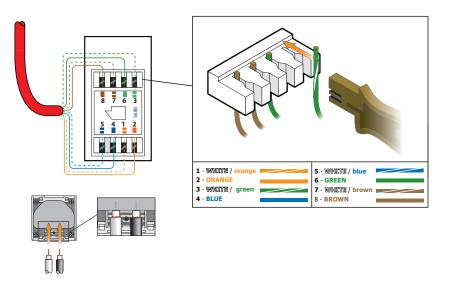
Ensure the core is fully pushed back into the IDC connector or it may result in no or a poor connection.
